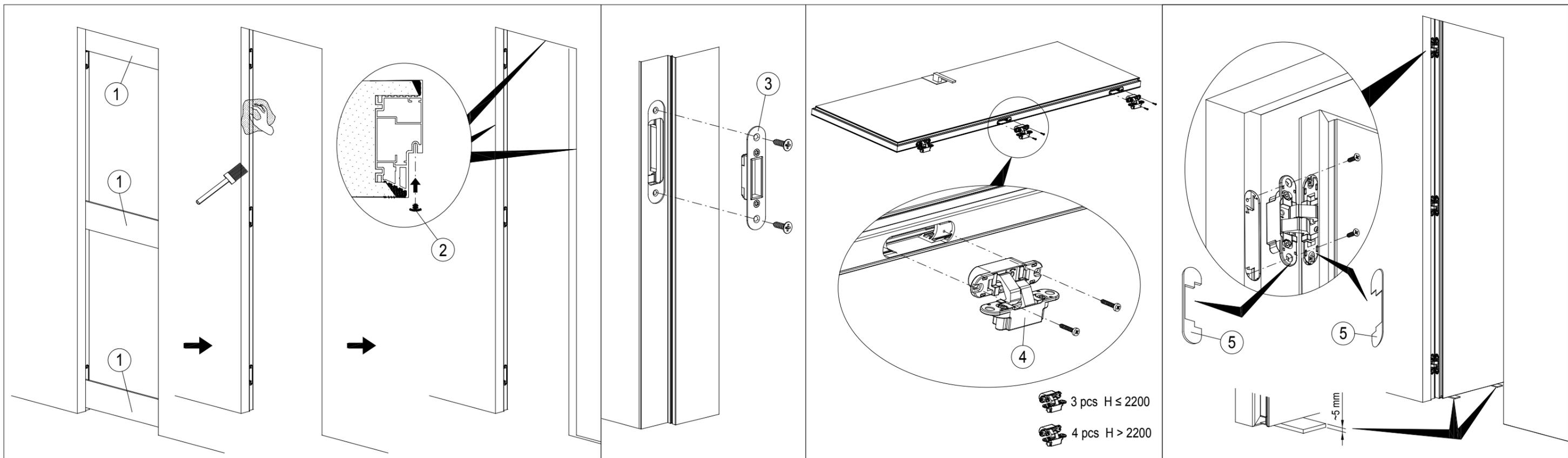
Remove the wooden spacers (1). Clean the aluminium frame. Apply a primer (e.g. cementite/undercoat). Proceed with the final painting. Install the sealing strip (2) on the frame. Secure the lock strike plate (3) to the frame. Install the hinges (4) on the door. Screw the door to the frame using shims (~5mm). Before moving the door, make sure there is no interference between the glass and the frame; if necessary, make adjustments by means of the hinges (4) and the jig (3). Fit the covers (5).
