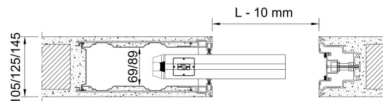
CONTROTELAIO ANTA UNICA "INTONACO"
